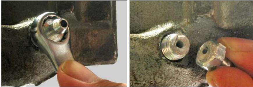
Initial situation: bleed screw has been broken off.
