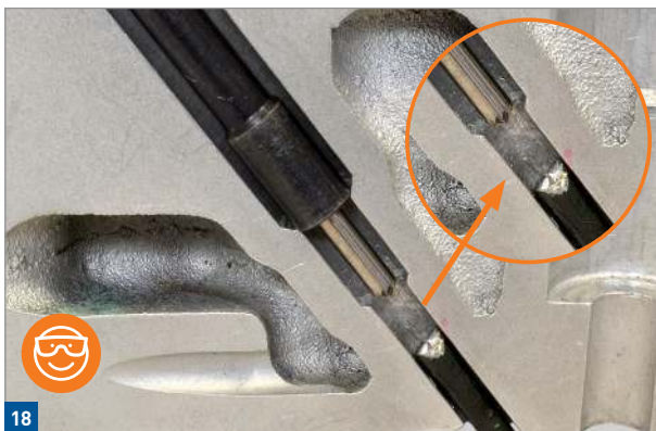
Cross section of the cylinder head
