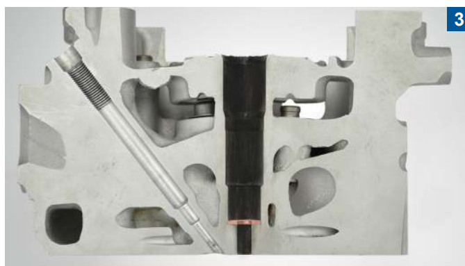
Cylinder head cross section with soiled injector shaft
