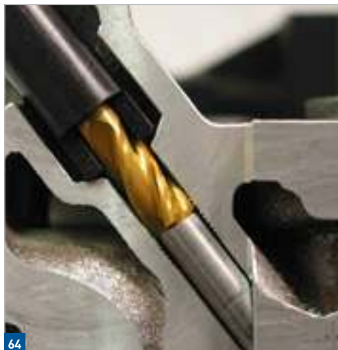
Glow plug bore in section
