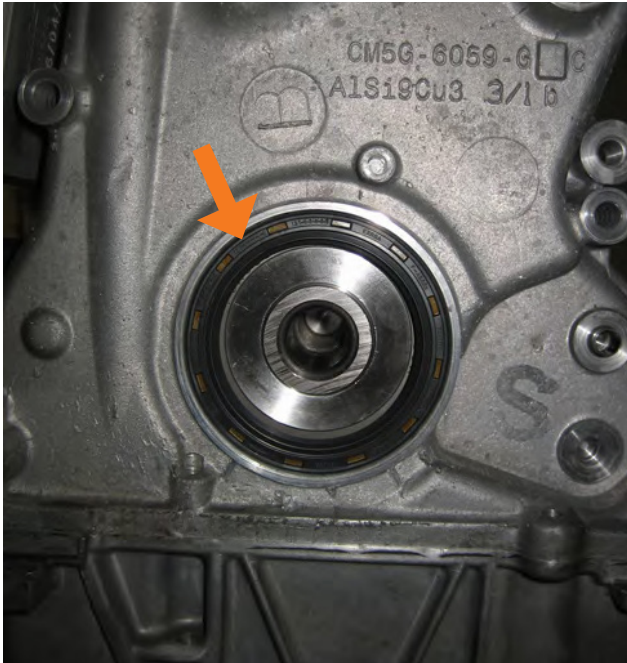
Fit a new crankshaft oil seal into the timing belt cover.
