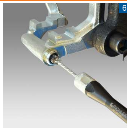
caliper sliding guide (slide pin bore)
