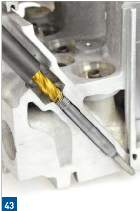
Cross section of the cylinder head and glow plug shaft
