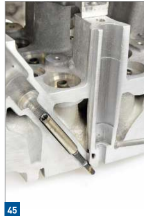
Cross section of the cylinder head and glow plug shaft
