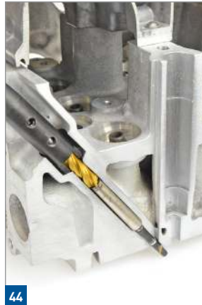
Cross section of the cylinder head and glow plug shaft
