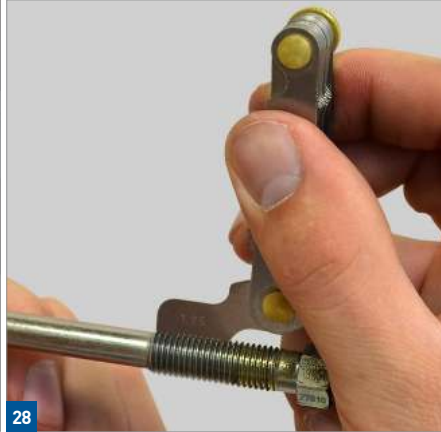
Check glow plug thread size M10x1 and pitch by measurement
