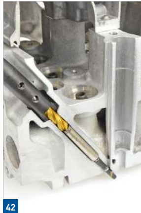
Cylinder head with glow plug bore in section
