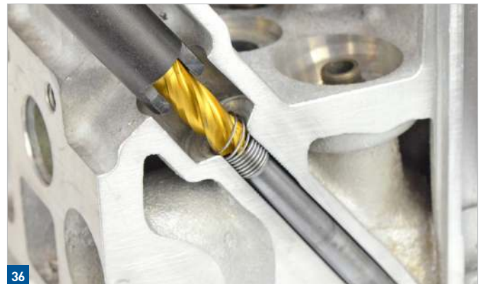
Cylinder head with glow plug bore in section
